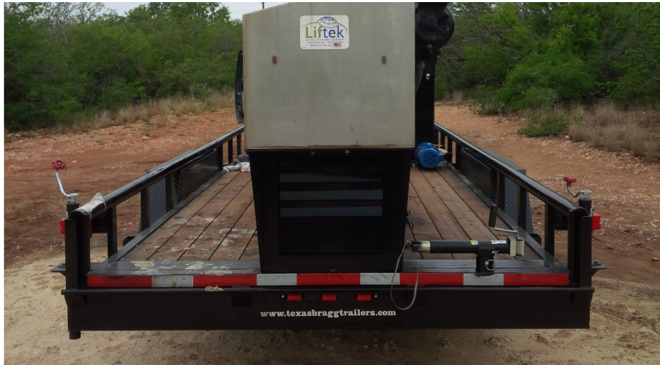
Figure 2 Oil Hound Rear View with Leveling Jacks
